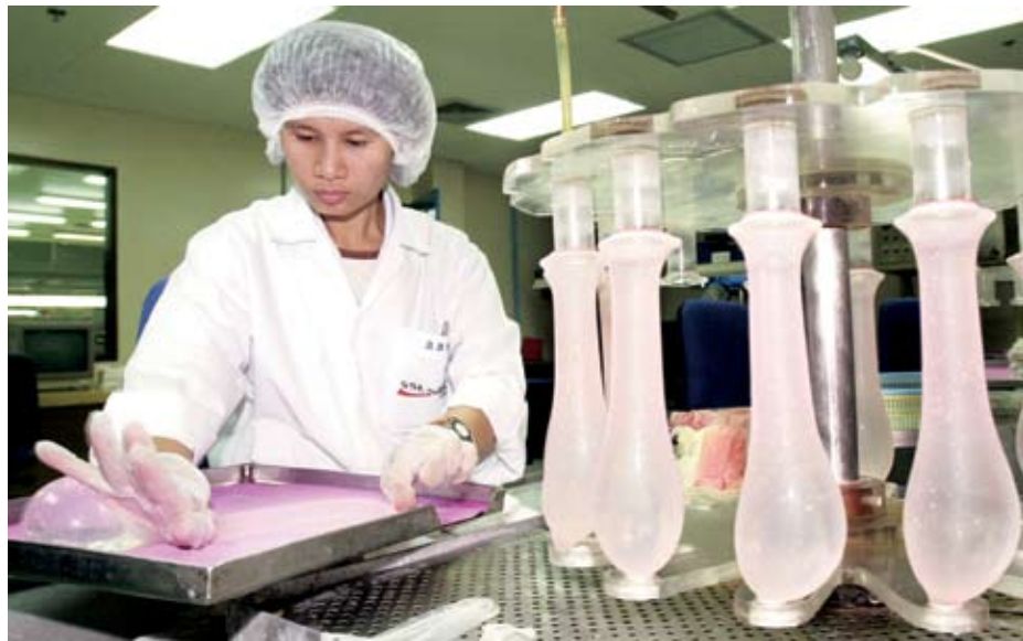
A technician at the Durex condom factory in Chonburi province, 70km south of Bangkok, makes a random test of condoms by putting in water to check for the leaking. Thailand is credited with bringing down the rate of HIV infection by 80 per cent after a massive awareness and condom distribution campaign in the early 1990s. Photograph by Sakchai Lalit/AP
